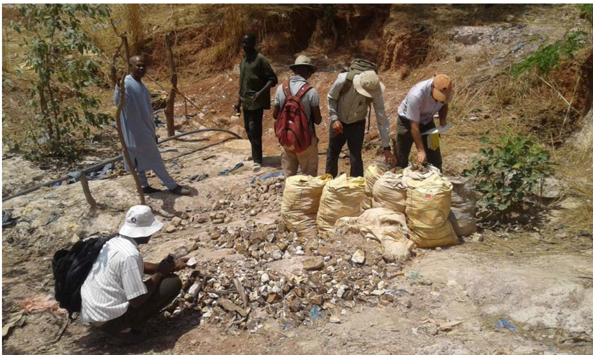
Figure 7: Mineralized quartz veins recovered from hand-excavated shafts ~20m in depth (example behind worker in green shirt where pipe enters ground) by artisanal workers.
