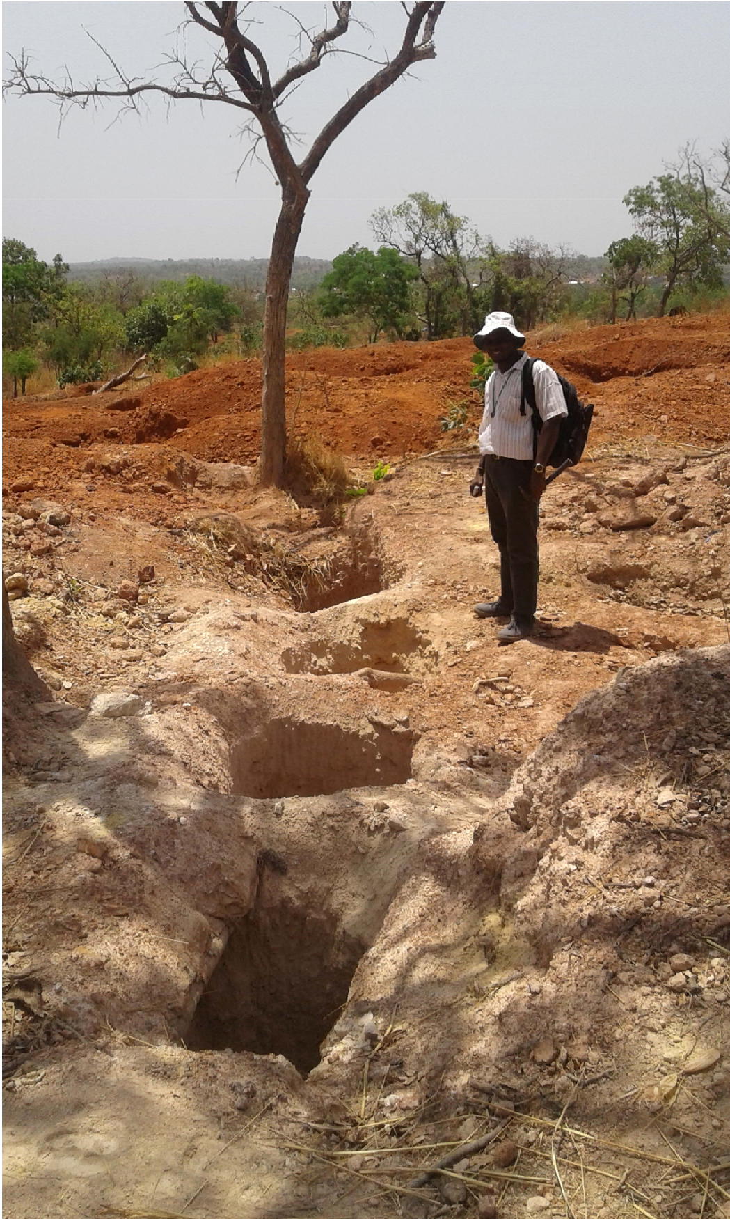
Figure 8: Artisanal working of kaolinitic saprolite follows linear north-south trend.
