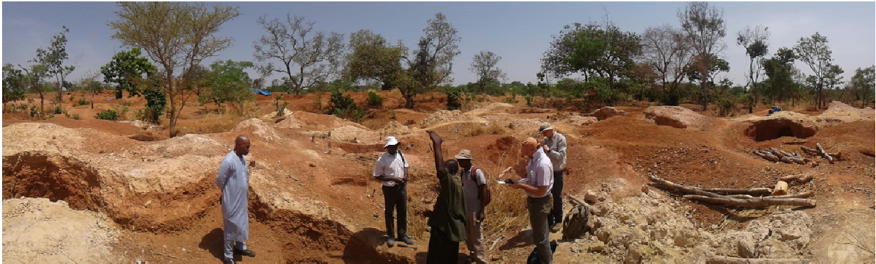
Figure 5: Artisanal pitting south of existing Resource at Yagbelen. Pits are aligned perpendicular to the strike of mineralized quartz veining, seen in abundance in spoil piles.
